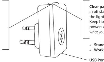
**Clear pairing history:** With the Bluetooth adapter in off state, press and hold the top button until the light alternately flashes red and blue quickly. Keep holding it until it flashes red twice and powers off. *Please do not do this unless you know what you are doing.*
